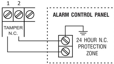
The tamper switch is Normally Closed while the keypad is secured on gang box. It is open when the keypad is removed from the gang box. To prevent sabotage, connect these terminals in series with a 24 hour N.C. protection zone of an alarm system if required.
