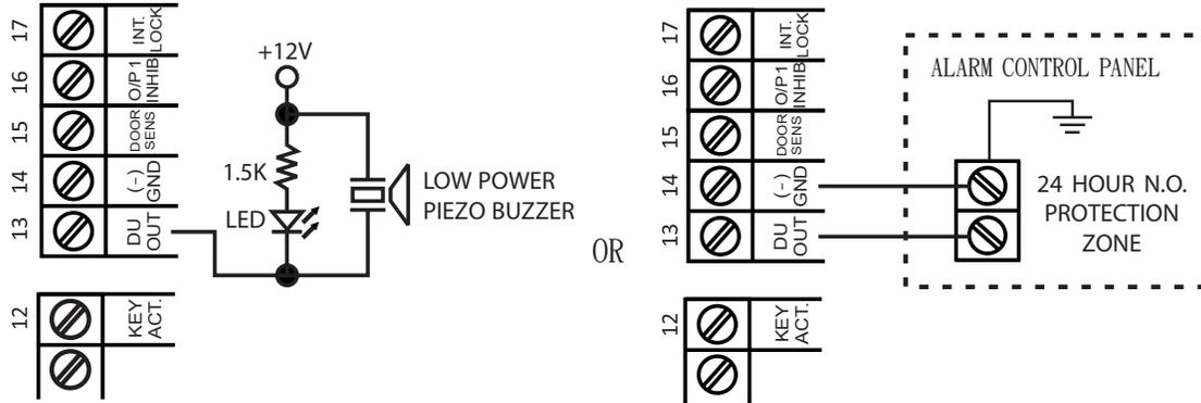
The Duress Output will switch to (-) ground when duress code is entered. You may use it to turn ON an LED lamp and / or small a buzzer to notify a guard; or connect it to a 24 hour Normally Open protection zone of an alarm system.
