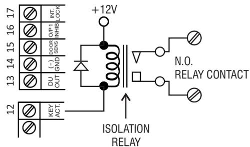
The Key Active Output will switch to (-) ground for 10 seconds whenever a key is touched. You may use it to turn ON an LED lamp and /or a small buzzer to notify a guard; or to energize a relay to switch ON lights or trigger an CCTV Camera to start recording.
