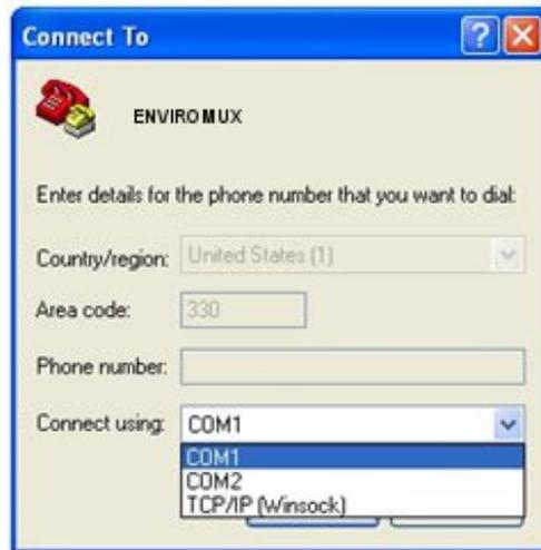
Figure 11- Configure COM port in HyperTerminal
