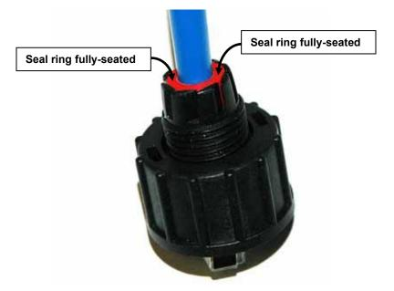
6. Plug the assembly into the socket on the ENVIROMUX-STS-O and secure the screw nut. Then apply the sealing nut and securely tighten.
