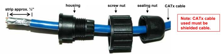
3. Terminate the CATx shielded cable with an RJ45 connector.
